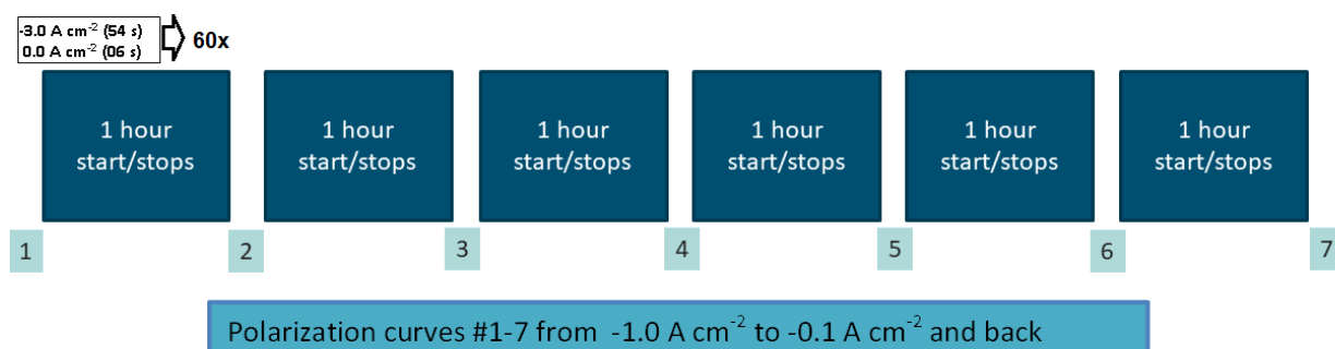
Figure 1. Schematic presentation of the ASLT procedure developed by PERMASCAND
