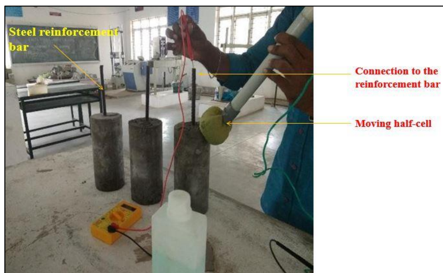
Figure 3. Typical Half-cell potential measurement arrangement
