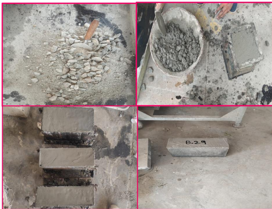
Figure 5. Casting of Conventional Block and LWC block
