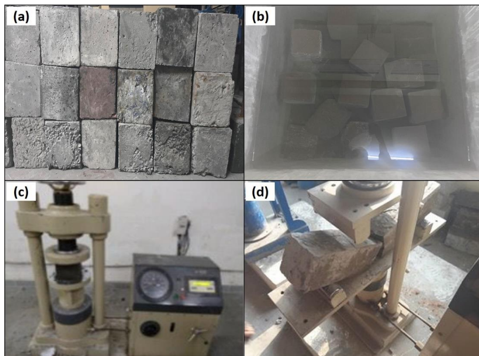
Figure 2. Digital photograph of (a) cast samples, (b) curing process, (c) compressive test and (d) flexural test being carried out on the samples
