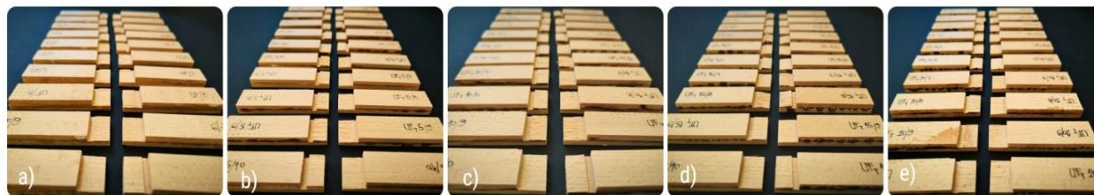
Figure 4. The failure zone of all sample groups: (a) cured pure UF, (b) UF cured with 5% tannin, (c) UF cured with 10% tannin, (d) UF cured with 15% tannin and (e) UF cured with 20% tannin
