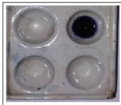
Figure 3. Testing of Sulphur by Lassaigne's test
