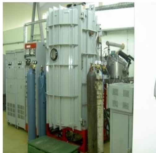
Figure 7 - PVD chamber (VU 1100) in Plasma facility
