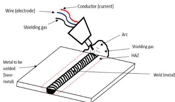
Figure 2. Gas metal arc welding process [15, 16]
