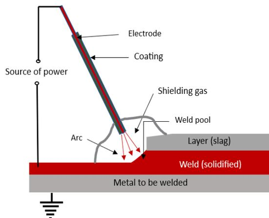
Figure 1. Schematic illustration of shielding metal arc welding [10]
