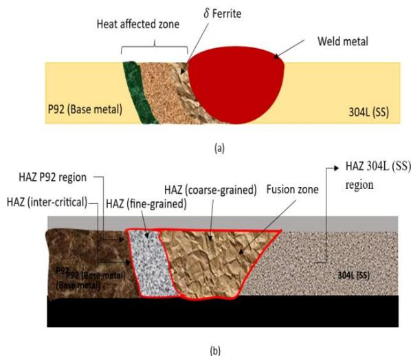
Figure 3 (a) Schematic illustration of different regions created in the dissimilar SS304 L and P92 welded joints. (b) A macrograph of the welded joint demonstrating the many zones created throughout the joint [23]
