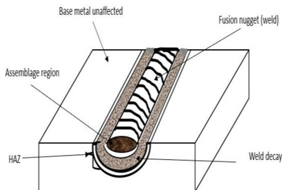
Figure 4. Schematic illustration of stainless steel's weld decay [25]
