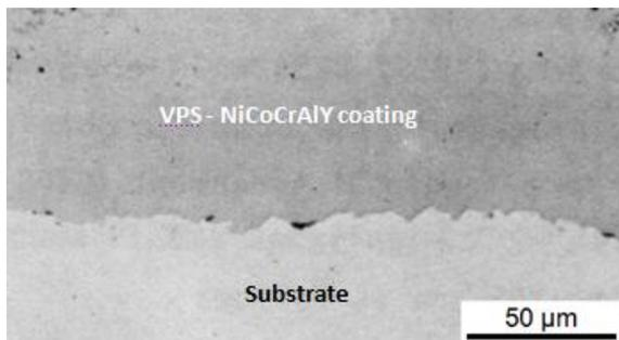
Figure 2. (OM) micrograph of VPS - NiCoCrAlY coating, left edge of the sample
