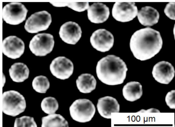
Figure 1. (SEM) Scanning electron micrograph of the NiCoCrAlY powder particles
