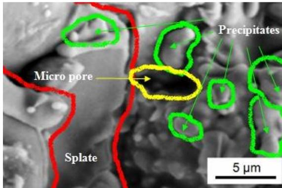
Figure 5. (SEM) Surface morphology of the VPS - NiCoCrAlY coating.
