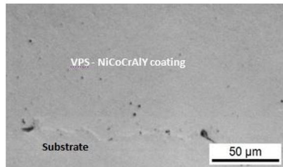
Figure 3. (OM) micrograph of VPS - NiCoCrAlY coating, mid-sample
