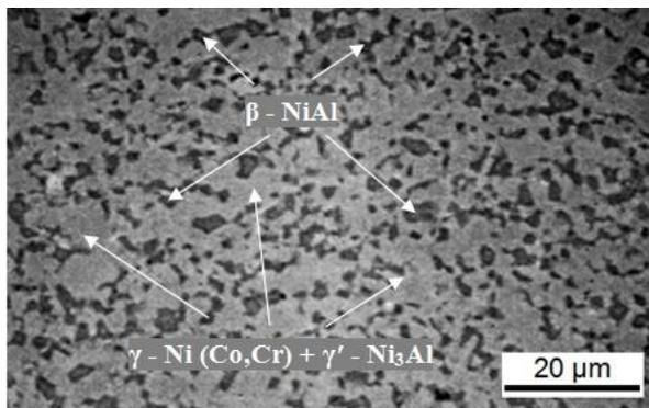
Figure 6. (SEM) micrograph of the etched microstructure of the NiCoCrAlY coating after heat treatment at 1150 °C/2 hours.
