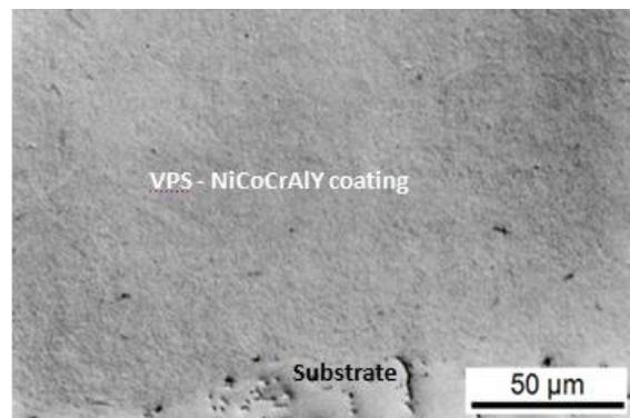
Figure 4. (OM) micrograph of VPS - NiCoCrAlY coating, right edge of the sample
