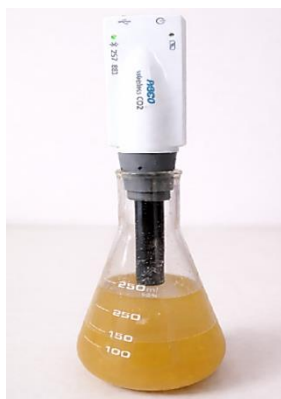
Figure 6. Experimental setup for \text{CO}_2 quantification
