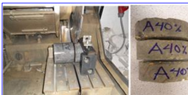
Figure 2. Preparation of samples (50mm thickness) for chloride diffusion test by cutting concrete cylinder by saw
