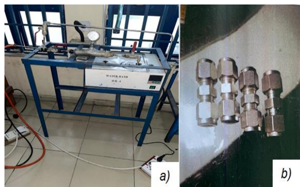
Figure 2. H 2 S and SO 2 adsorption equipment, (a) Experimental setup for evaluation of H 2 S and SO 2 adsorption capacity (b) Reactors for storing adsorbents
