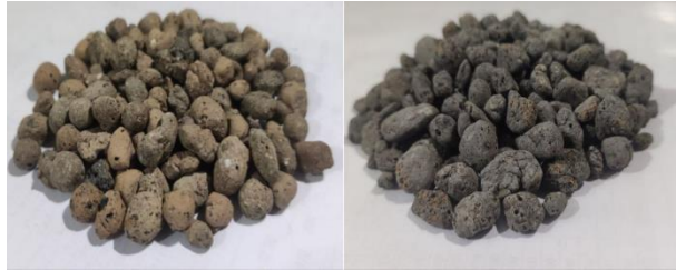
Figure 1. Two different types of LECA from left (LL), and from right (LH)
