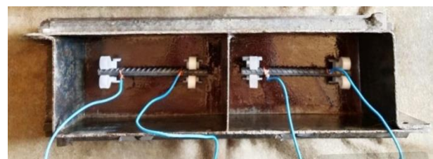
Figure 3. Molds and rebar for accelerated corrosion
