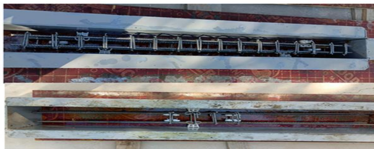
Figure 2. Details of the steel reinforcement (a) flexural, (b) shear, (c) moulds for beam Specimens
