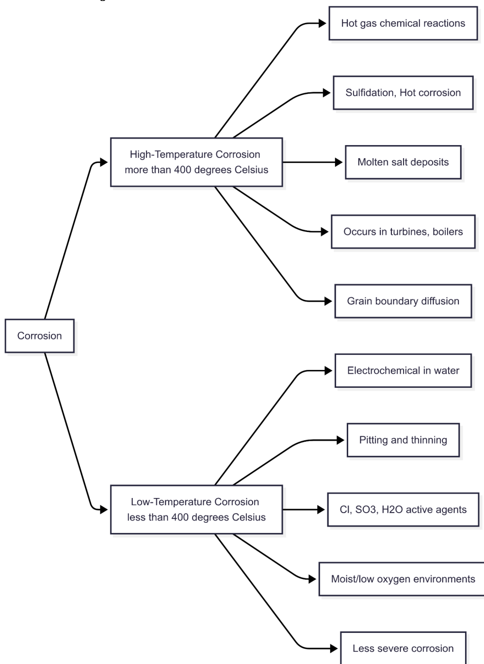
Figure 1. Corrosion at low and high temperature
