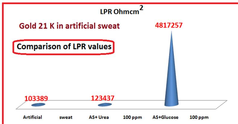
Figure 5. Comparison of LPR values of Gold 21K immersed in various test solutions
