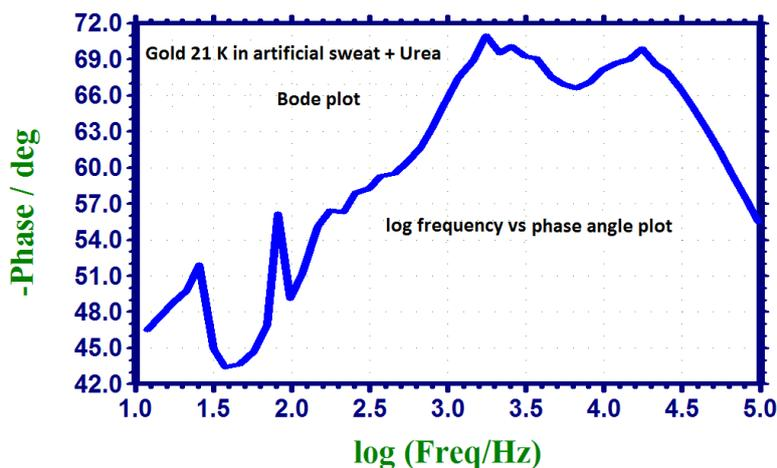
Figure 12. Log frequency vs. phase angle plot of Gold 21K immersed in artificial sweat (AS) + Urea
