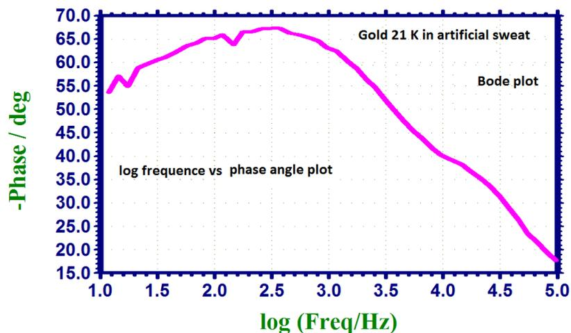
Figure 9. Log frequency vs. phase angle plot of Gold 21K immersed in artificial sweat (AS)
