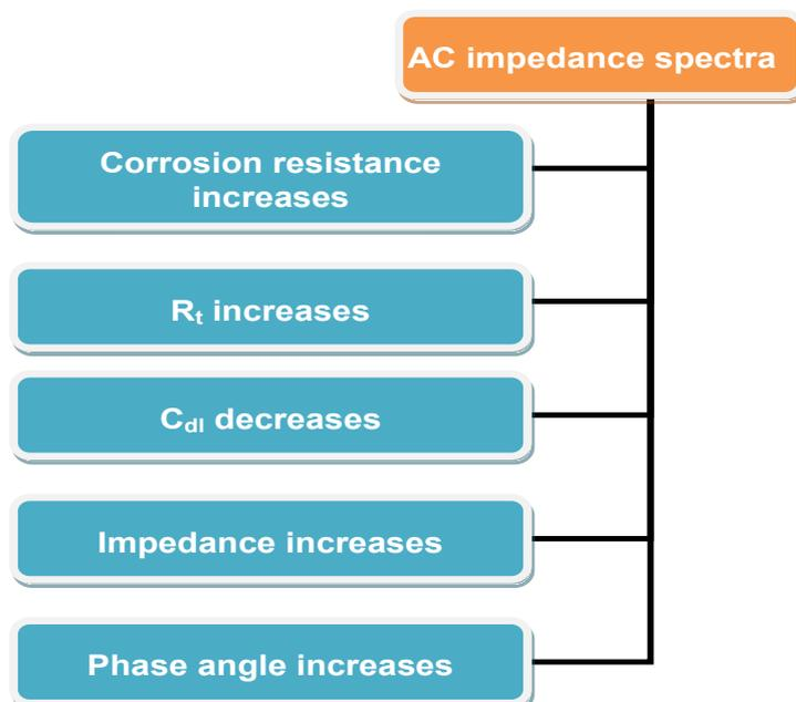
Scheme B. Correlation among corrosion parameters in AC impedance spectra
