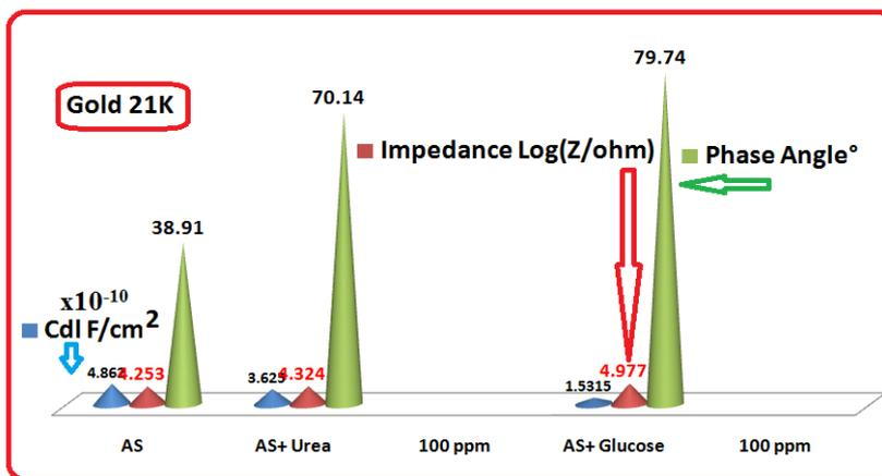
Figure 17. Comparison of corrosion parameters of Gold 21K immersed in various test solutions
