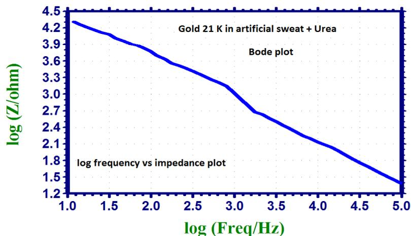
Figure 11. Log frequency vs. impedance plot of Gold 21K immersed in artificial sweat (AS) + Urea
