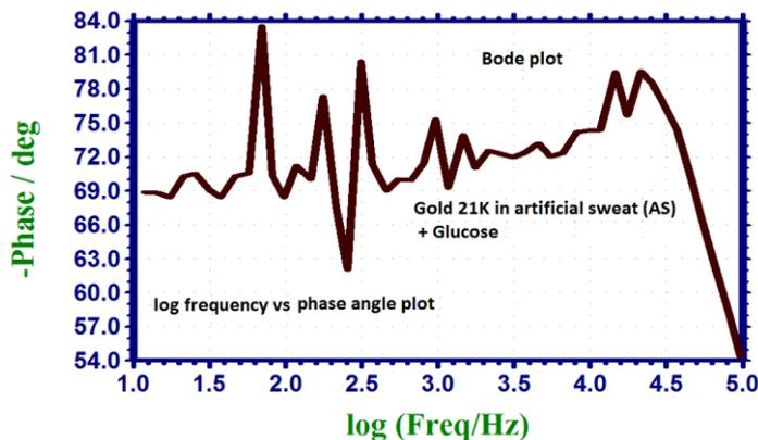
Figure 15. Log frequency vs. phase angle plot of Gold 21K immersed in artificial sweat (AS) + Glucose
