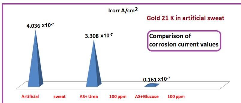
Figure 6. Comparison of corrosion current values of Gold 21K immersed in various test solutions
