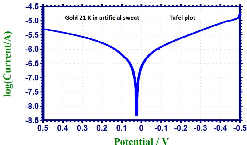
Figure 1. Polarization curve of Gold 21K immersed in artificial sweat (AS)
