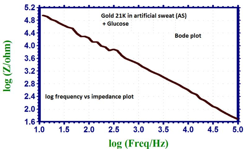
Figure 14. Log frequency vs. impedance plot of Gold 21K immersed in artificial sweat (AS) + Glucose
