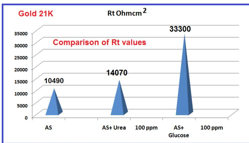
Figure 16. Comparison of  $R_t$  values of Gold 21K immersed in various test solutions
