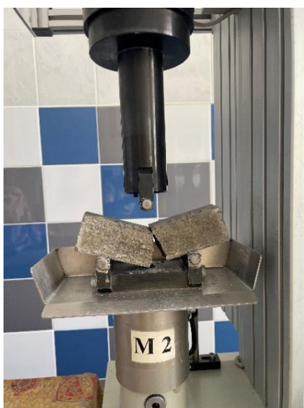
Figure 8. Determining of flexural strength
