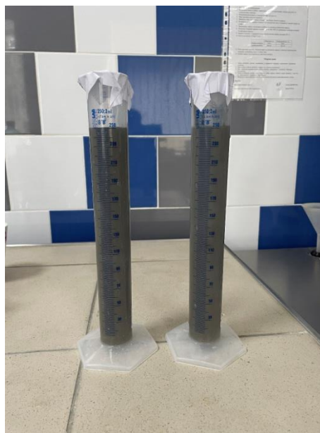
Figure4. Determination of water separation
