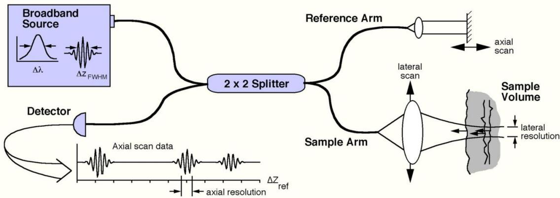
Figure 3. OCT experimental setup
