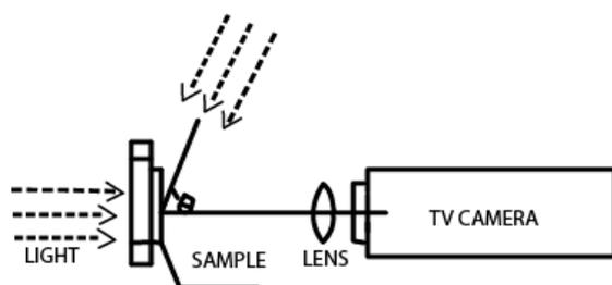
Figure 2. Geometrical arrangement to obtain the images of the woven fabric
