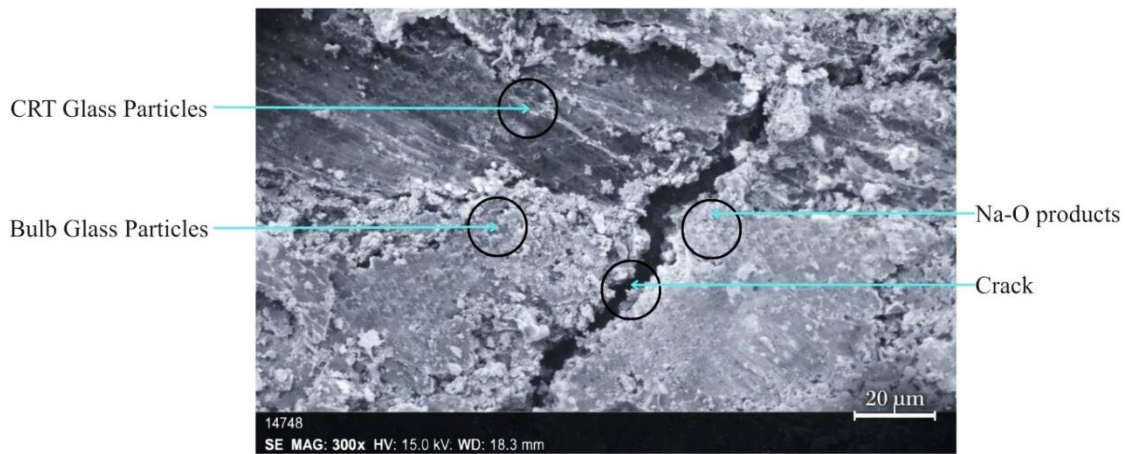
Figure 11: Glass (extracted from waste bulbs and CRT)epoxy composite SEM picture that has been alkali treated (x300)
