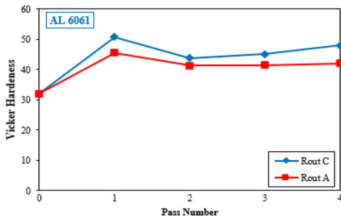
Figure 7. Micro hardness test for Al 6061 with annealing process after first pass
