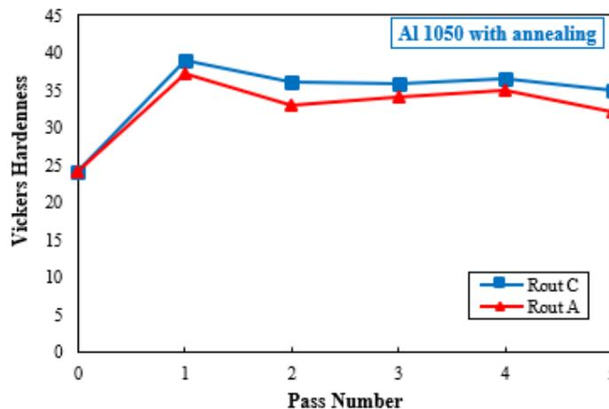
Figure 8. Micro hardness test for Al 1050 a) at ambient temperature, b) at annealing process
