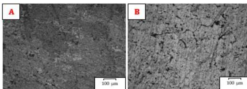
Figure 2. Optical micrograph for Al 6061 rout C a) first pass b) fourth pass
