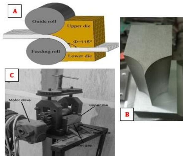
Figure 1. a) Schematic illustration of the ecar device, b) Die with angle  $115^\circ$ , c) The machine device used with die
