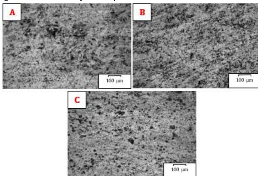
Figure 3. Optical micrograph for Al 1050 rout C a) first pass. B) six passes without annealing.
