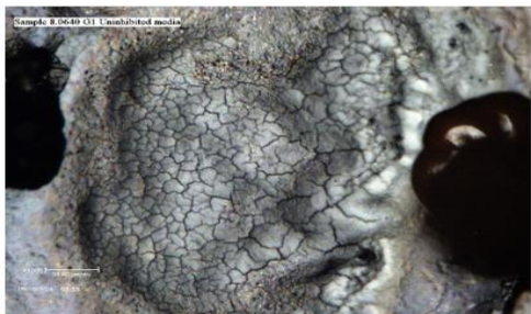
(c) 0g (uninhibited) after 20 days (etched)
