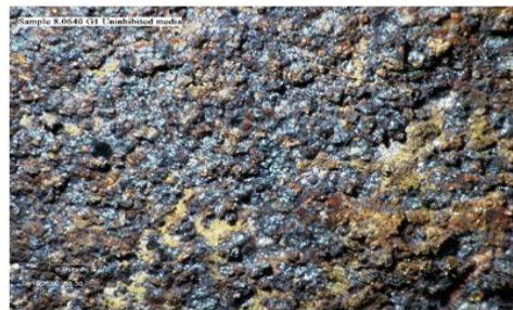
(d) 0g (uninhibited) after 20 days (unetched)
