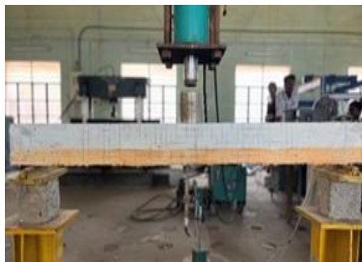
Figure 5. ECC layered at 50mm in the tension zone of beam
