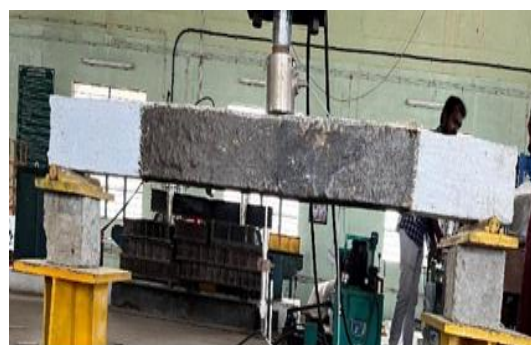
Figure 6. Control beam wrapped with BFRP sheet
