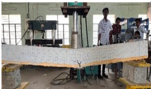
Figure 4. ECC layered at 20mm in the tension zone of beam
