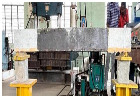
Figure 7.20 mm ECC layered retrofitted by BFRP
