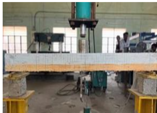
Figure 5. ECC layered at 50mm in the tension zone of beam
