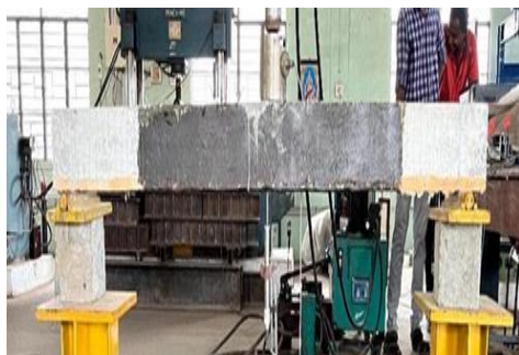
Figure 7. 20 mm ECC layered retrofitted by BFRP
