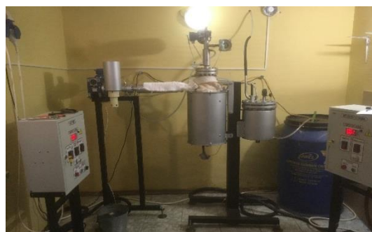
Figure 1. The equipment for pyrolysis of polyolefins
