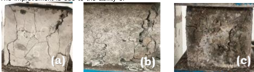
Fig. 17 Cube Compression test of RAC and fiber reinforced RAC (a) Control (b) Single fiber RAC (c) Hybrid Fiber RAC
