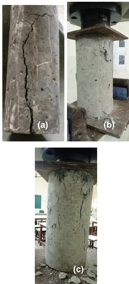
Figure 8. Uniaxial compression failure (a) Control concrete (b) RAC 25% (c) RAC 50%
