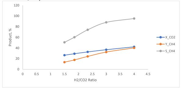
Figure 6. Effect of H<sub>2</sub>/CO<sub>2</sub> ratio on CO<sub>2</sub> conversion, CH<sub>4</sub> selectivity and yield at 50 bar pressure and 500°C temperature
