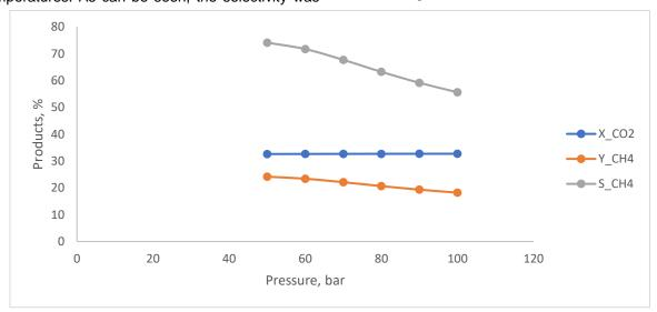
Figure 5. Effect of pressure on CO<sub>2</sub> conversion, CH<sub>4</sub> selectivity yield at 500°C, and H<sub>2</sub>/CO<sub>2</sub> ratio of 2.33
