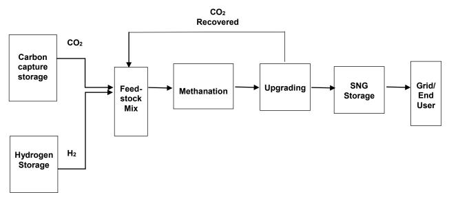
Figure 1. Block diagram of the synthetic methane production process
