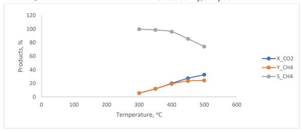
Figure 4. Effect of temperature on CO<sub>2</sub> conversion, CH<sub>4</sub> selectivity and yield for 50 bar pressure and H<sub>2</sub>/CO<sub>2</sub> ratio of 2.33
