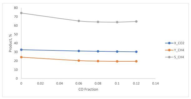
Figure 7. Effect of CO fraction in feed on CO<sub>2</sub> conversion, CH<sub>4</sub> selectivity, and CH<sub>4</sub> yield
