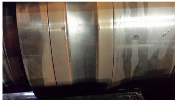
Figure 6. Surface of an HSS ring after use [27, 28]
