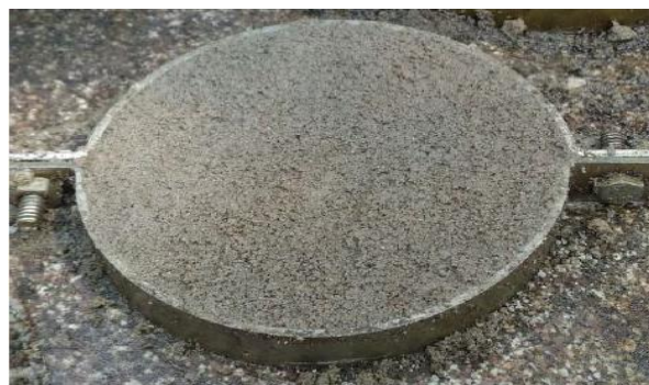
Figure 4. Casting of circular specimens for thermal conductivity
