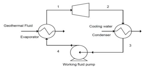
Figure 1. The working principle of the ORC system Slika 1. Princip rada ORC sistema
