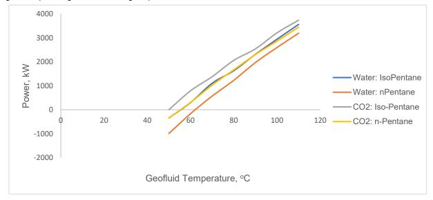
Figure 10. Effect of Geofluid on power production using water and CO<sub>2</sub> geofluids Slika 10. Uticaj Geofluida na proizvodnju energije korišćenjem vode i CO<sub>2</sub> geofluida
