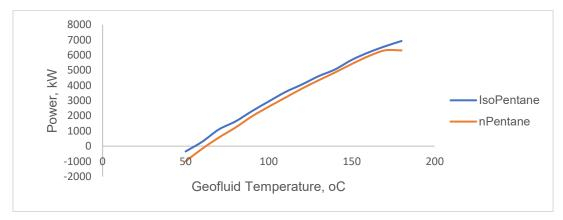
Figure 4. Effect of geofluid temperature on power produced using water as geofluid at 80 kg/s Slika 4. Uticaj masenog protoka na proizvodnju energije korišćenjem vode kao geofluida na 100 °C
