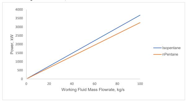
Figure 6. Effect of mass flowrate on power production using water as geofluid at 100°C Slika 6. Uticaj masenog protoka na proizvodnju energije korišćenjem vode kao geofluida na 100°C
