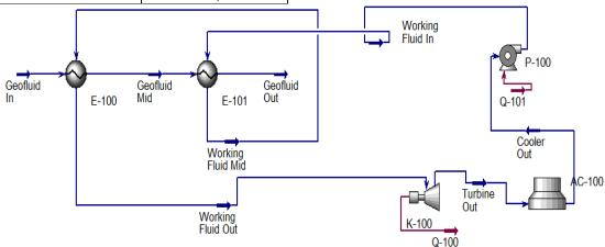
Figure 3. Process flow diagram (PFD) of the geothermal binary ORC system Slika 3. Dijagram toka procesa (PFD) geotermalnog binarnog ORC sistema
