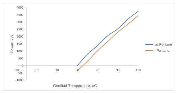
Figure 7. Effect of geofluid temperature on power produced using CO<sub>2</sub> as geofluid at 80 kg/s Slika 7. Uticaj temperature geofluida na snagu proizvedenu korišćenjem CO<sub>2</sub> kao geofluida pri 80 kg/s
