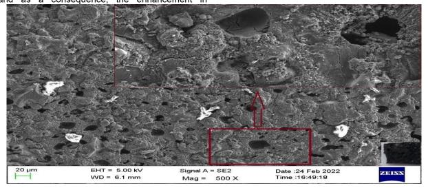
Figure 3. SEM image of Choline acetate (1.5gm) reinforced PVC-PVP-50%PPy Film (inset shows the magnified view) (c)Photographic image of film
