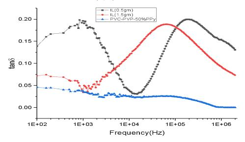
Figure 5. Variation in tand with frequency for Choline Acetate reinforced PVC-PVP-50%PPy film Slika 5. Varijacija u tand sa frekvencijom za PVC-PVP-50%PPi film ojačan holin acetatom
